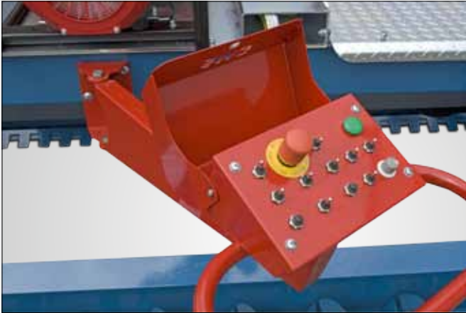
Pivotable control panel
