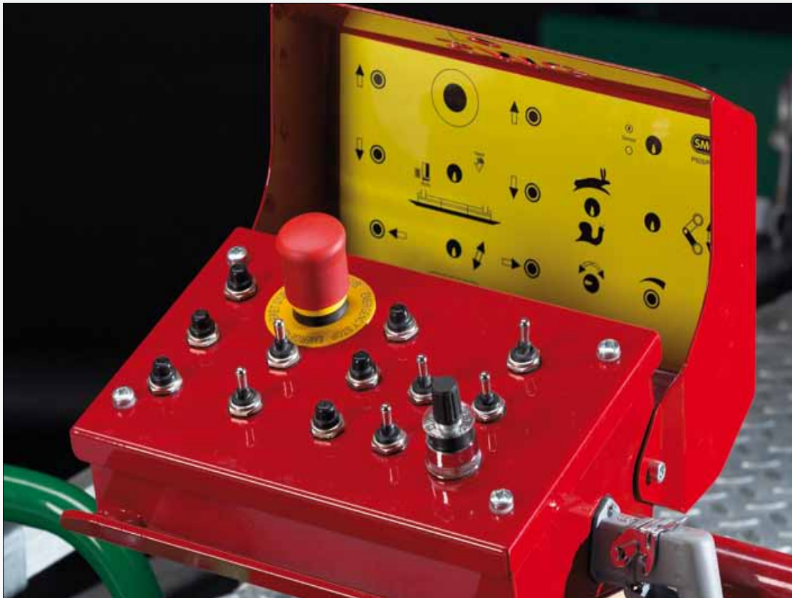
Control panel, installed on both sides, all operating functions including curve control integrated (P928/P936)
