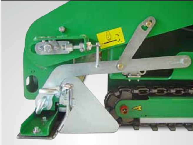
Electrical heated screed, adjusting spindle for the grade setting, material limiter
