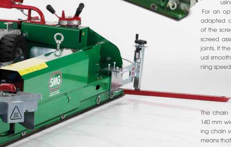
P928 with comfort seat, automatic levelling device and Hot Trowel
