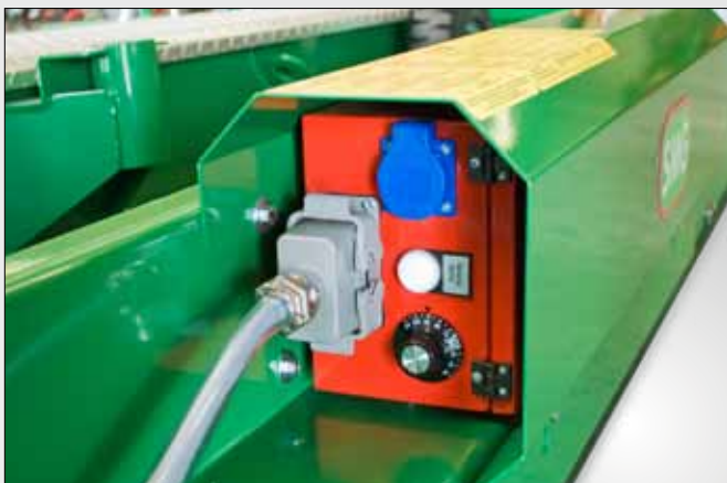
Screed heating with thermostat and additional 220 V power supply, e.g. for HotTrowel
