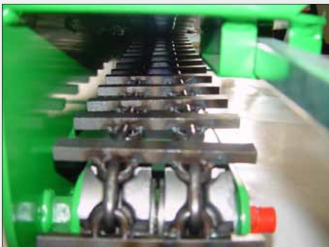
Wide chain drive unit (140 mm) for safe traction, on all kinds of subbase constructions
