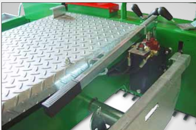
Additional hand pump for the manual up/down lifting of the machine
